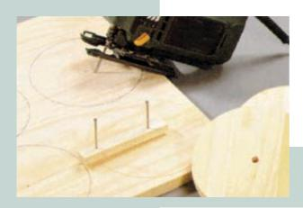
is a tip when gluing the two washers required for each wheel: drill the bores first, then you can simply slide the washers onto one axle and press together firmly with G-clamps without the parts being displaced.
