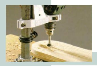
When screwing the base plate (3) onto the rear wall, the screw heads underneath may remain visible. Where the chipboard screws are inserted near the edge, for example with the axle bearings (6), pilot drilling must be carried to prevent the wood from chipping. To produce the different bores for the steering axle (10) and wheel axles, a drill stand is indispensable. Use only top quality drill bits that guarantee a really clean cut. Here
