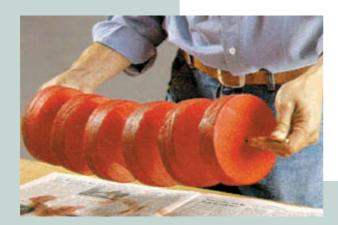
A small amount of candle wax applied to the aluminium axle guarantees particularly smooth running of the wheels. The trailer is assembled according to the same procedure as the playmobile. Also in this case there are only flush screw connections covered by wooden dowels.
