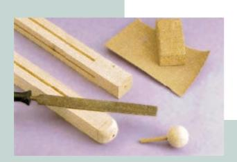
Now cut the eight frame strips and the four side walls to size. Fit a 6-mm straight bit onto your router. Now use the router to route a 10-mm deep groove in the centre of the posts and frame strips. The distance between the frame strips and end of post is 50 mm at the top, and 20 mm at the bottom.
