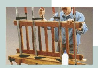
First, mark the positions of the slots on the workpieces. Now the appropriate straight bit is inserted in the router. At the starting point of every slot, the router plunges into the wood, the workpiece is then pushed along the stop until the slot end is reached. This task can be made easier by clamping two auxiliary stops on to the base plate of
