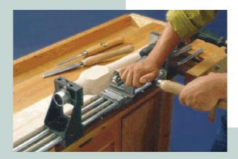
Making the fuselage is the first step. A  $60 \times 60$  mm squared timber is dressed to produce a 50 mm long taper at the front. 70 mm of the squared timber remain and the rear section is also tapered slightly. At the front, the position of the engine for the double-decker can also be marked by an appropriate notch.
