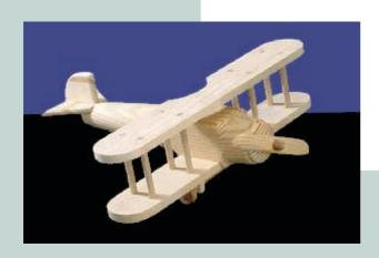
First bevel the moulded blank with a rasp, round off the edges and rework with sanding paper. A 6-mm piece of squared timber serves as a propeller axle.
