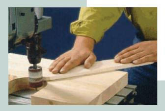
Then the drill stand is used to produce the holes for supporting the bearing surface braces. When both bearing surfaces have been glued to all eight bearing surface braces, the chassis is built and glued below this in the centre.
