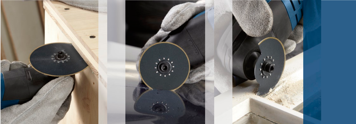
Cutting wood with nails.
