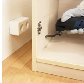
Cutting a recess in furniture components, e.g. to enable access to a mains socket.
